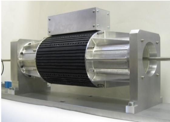
Fig. 2. Prototype LEA on test rig
