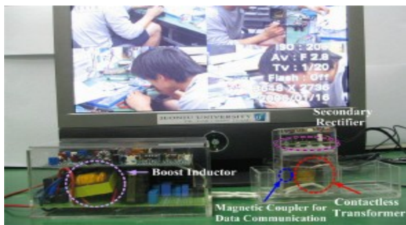
Fig. 15. Prototype of a contact-less power supply for the photovoltaic power generation system LCD TV
