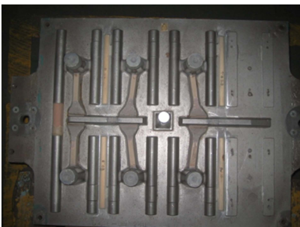
Fig. 1. Metal pattern for bar test castings.
