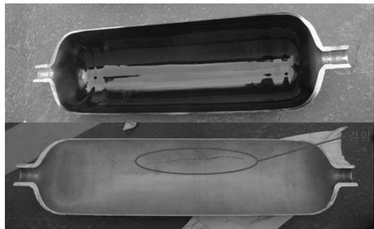
Fig. 4. Penetrant test result for inner liner of Type 3 cylinder
