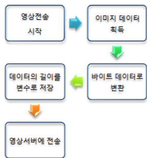
[Fig. 9] Processing of Video Transfer for Receiving
