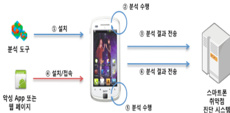
[Fig. 9] Implemented System Architecture
