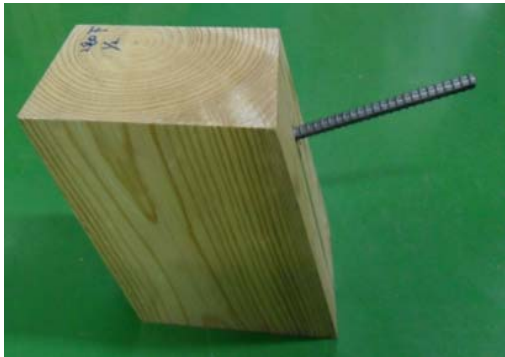
Fig. 2. Prepared wood anchored with steel rebar.
