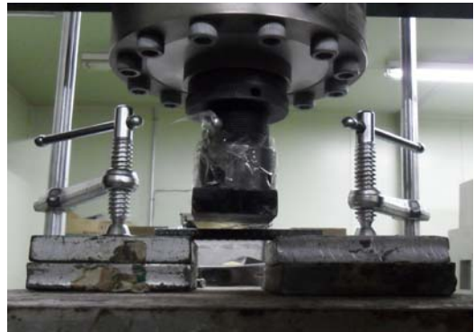
Fig. 4. Shear test of steel rebar.
