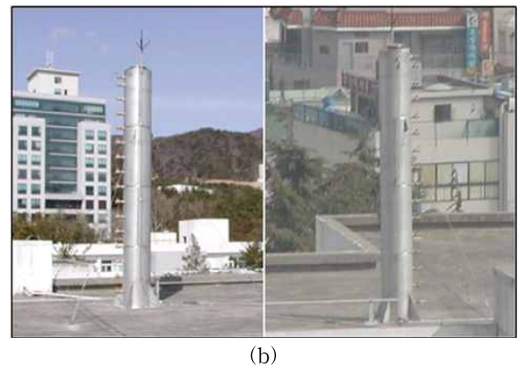
Fig. 1. Experimental Pipeline System for Generating and Measuring Waterhammer (a); pictures for tanks A and B (b).
