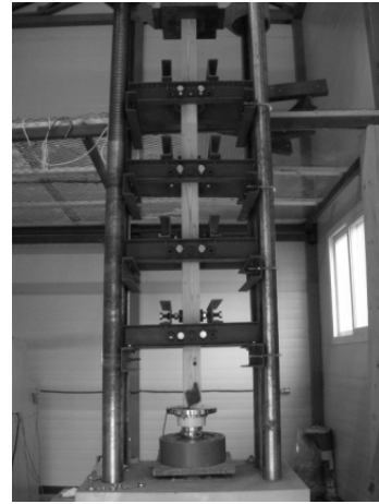
Fig. 2. Compressive strength test of specimens.
