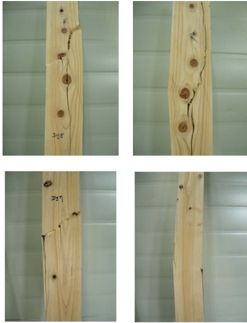
Fig. 7. Failure mode of compressive strength test.
