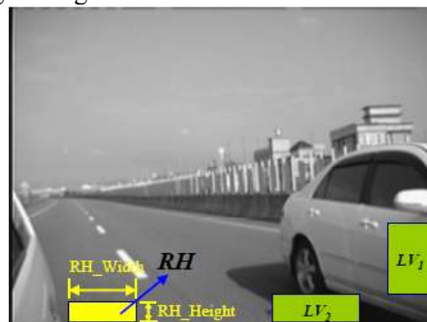
Fig. 12. The region checked in order to detect a vehicle in the neighboring lane
