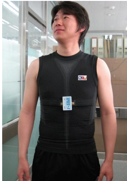
Fig. 3. Wearable shirts with IFUS-1 node and ECG/accelerometer sensors.
