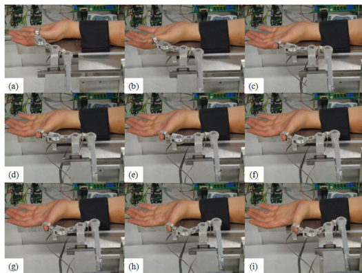
Fig. 8 Characteristic test for flexibility rehabilitation exercise of thumb using thumb rehabilitation robot
