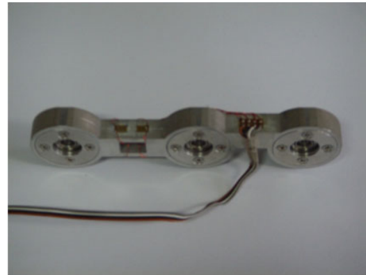
Fig. 5 Photograph of manufactured thumb force sensor
