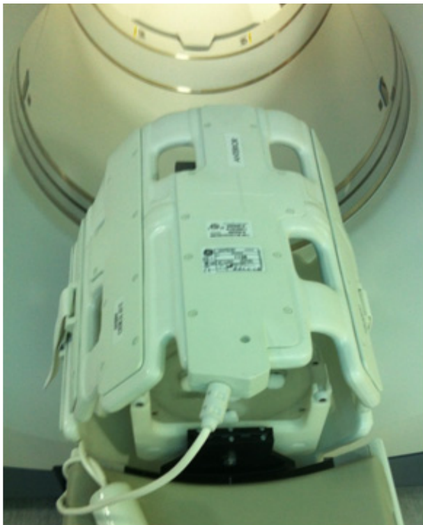
Fig. 1. Phantom was surrounded by MR Torso Coil.
