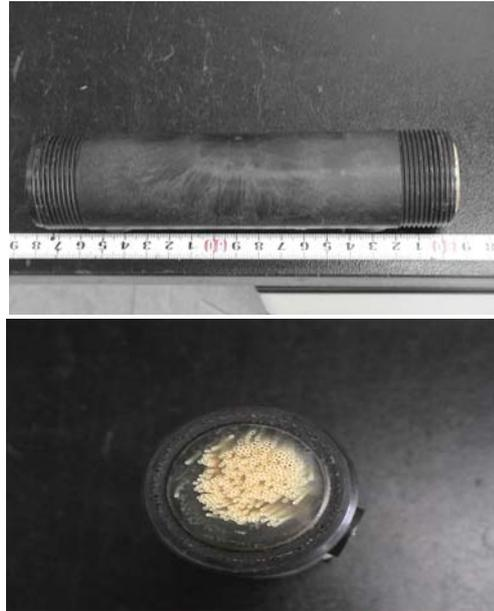
Fig. 12. Photographs of sample module (Size of sample :  $\phi$  1.5 inch  $\times$  L7 inch).
