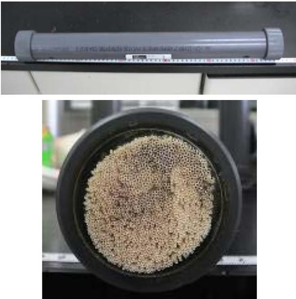
Fig. 11. Photographs of sample module (Size of sample :  $\phi$  2 inch  $\times$  L22 inch).
