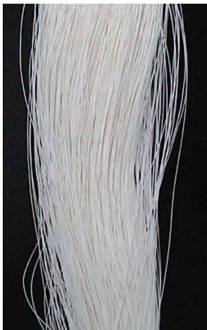
Fig. 7. Photograph of hollow fiber membrane in this study.
