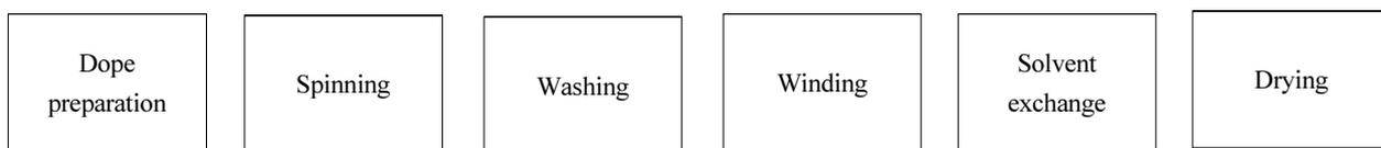
Fig. 6. Procedure of hollow fiber preparation.
