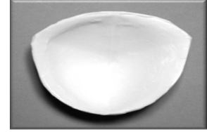
[Figure 10] Pad by casting
