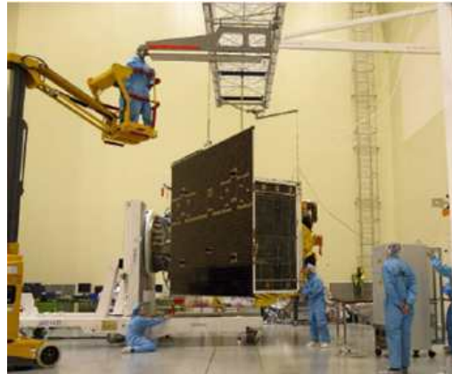
Fig. 2. Solar array deployment test
