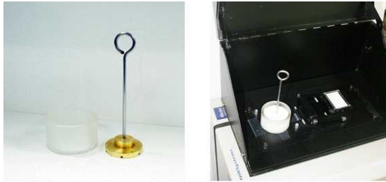
Fig. 2. Sample cell, reflectance plate(left) and horizontal type spectrophotometer(right) for reflectance spectra measurements.
