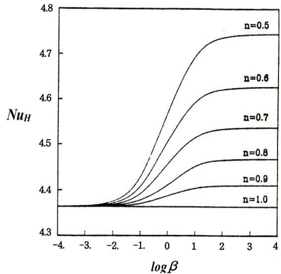
Fig. 3 Variation of Nusselt number (CHF) with shear rate parameter ( $\beta$ ) for shear-thinning fluids in a circular conduit
