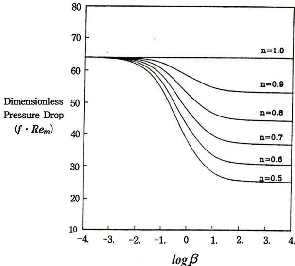
Fig. 2 Variation of dimensionless pressure drop with shear rate parameter ( $\beta$ ) for shear-thinning fluids in a circular conduit
