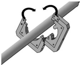
Fig. 3 Assembling procedure for the adapter on a shaft
