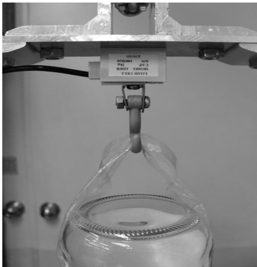
Fig. 1 Weight measurement using load cell
