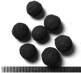
Fig. 3. Picture of pellets made from coal tailings and iron oxide (10%).
