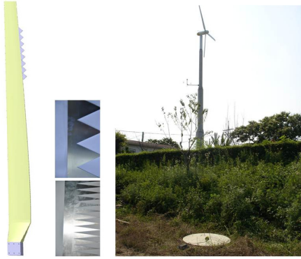
Fig. 9 The manufactured low noise serrated trailing edged blade and acoustic field test
