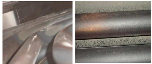
Fig. 7 Fly ash erosion on the primary reheat tube
