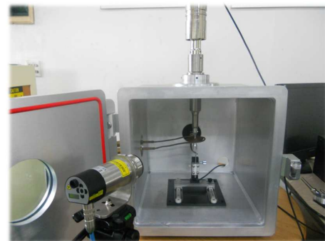
Fig. 14 System for ultrasonic fatigue test at high temperature
