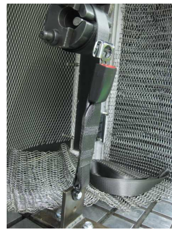
Fig. 3 Tensile performance test
