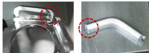
Fig. 4 Damaged DLT device
