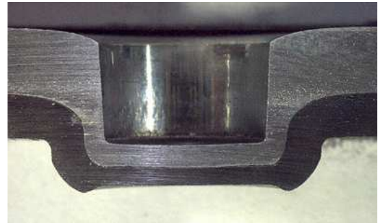
(a) Insufficient undercut
