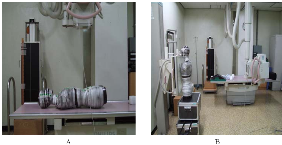
Fig. 1. Set up of test equipment at supine (a) and erect (b) positions of the Rando Man Phantom.
