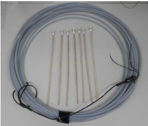
Fig. 2 Experimental bobbin probe for variation of coil winding number
