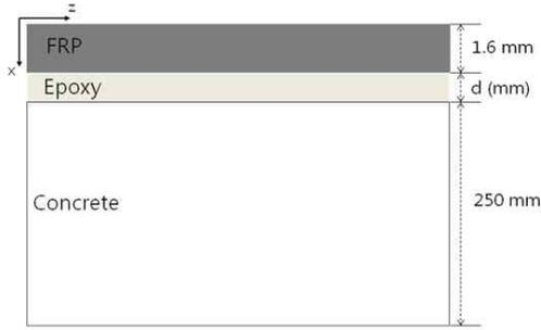
Fig. 1 FRP-epoxy-concrete model
