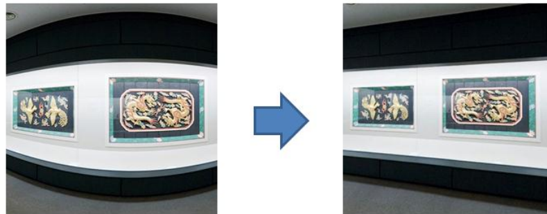
Fig. 3. Example of correcting fisheye distortion for a training image.
