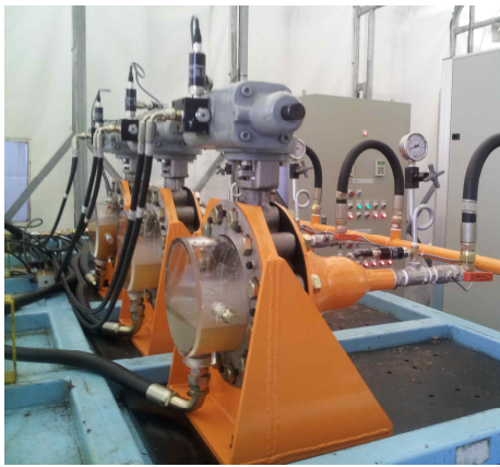
Fig. 7 The view of butterfly valve test equipment with 3 sets after 1st modification
