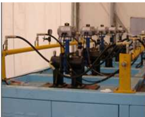
Fig. 3 Butterfly valve life test equipment before modification
