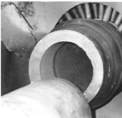
**Fig. 1** Example of weld section cutting damage by residual stresses in main steam pipe of power plant
