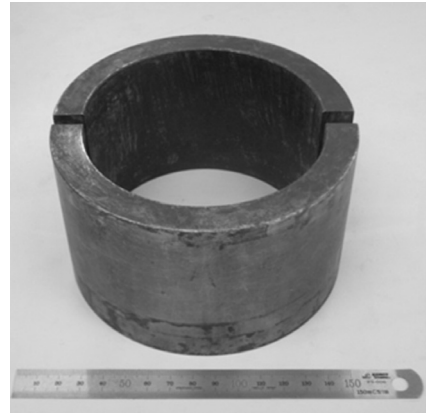
Fig. 3. Aluminum mold and cylindrical molding frame for circular replicas of the gneiss joint.
