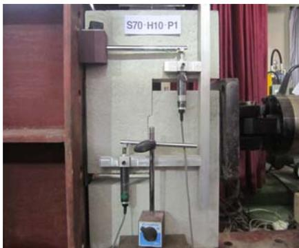
Fig. 7 Detail of displacement measurement
