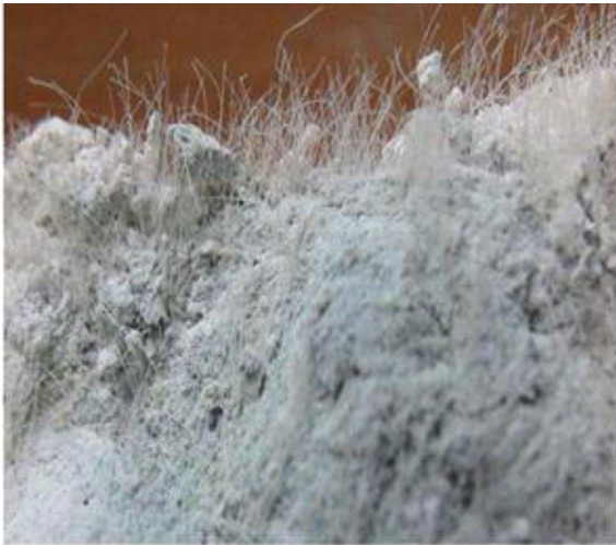
Fig. 9 Typical fiber dispersion of PVA fibers in cracked section
