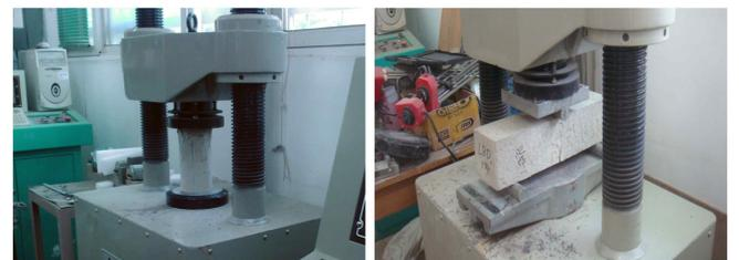
**Fig. 3** Compressive and flexural strength test
