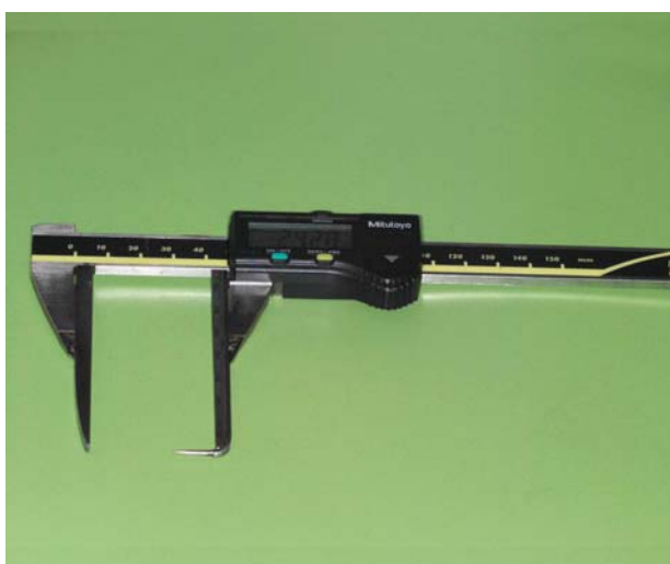
Fig. 3. A modified digital caliper to measure distance between landmarks located in concave surface.
