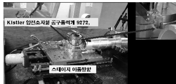
Fig. 9 Function measurement between cutting force and strain-gauge
