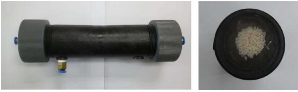
Fig. 2. Photograph of the test module and housing for hollow fiber membrane.
