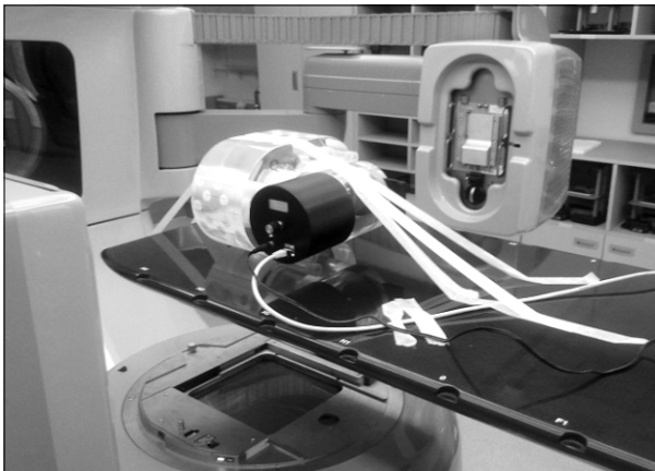
Fig. 1. QUASAR programmable respiratory motion phantom (Moudus Medical Device Inc. CANADA).
