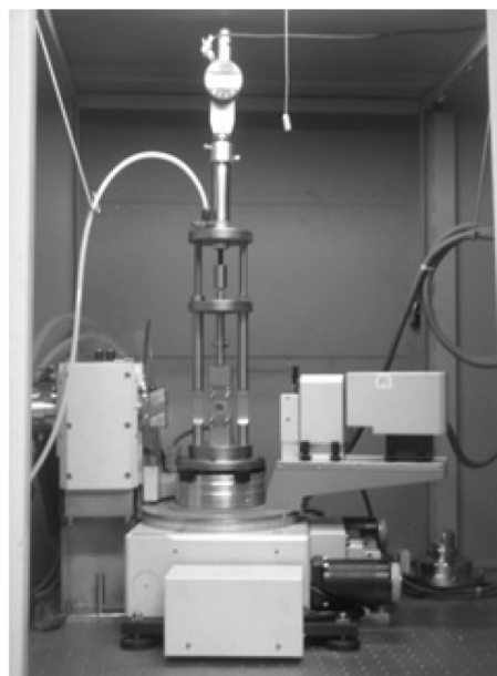
Figure 1. Creep device attached to X-ray diffractometer.
