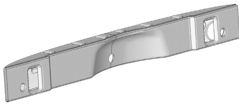
(a) With SPFC780 material (closed section)
