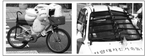
(a) Bicycle & Dummy (b) Vehicle Fig. 1 Bicycle and vehicle for crash test
