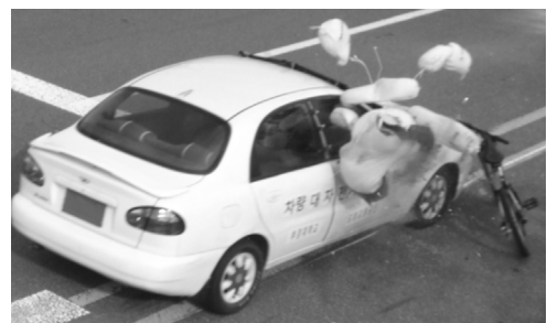
Fig. 2 Crash experiment of vehicle and bicycle
