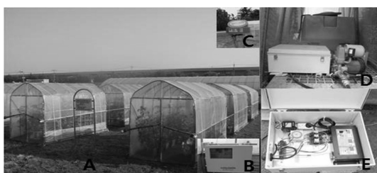
Fig. 1. View of experimental small greenhouse (A), ventilation controller (B), rain sensor (C), irrigated water tank (D), automatic irrigation controller (E).
