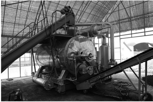
Fig. 2. Picture of the plug media sterilizer system.
