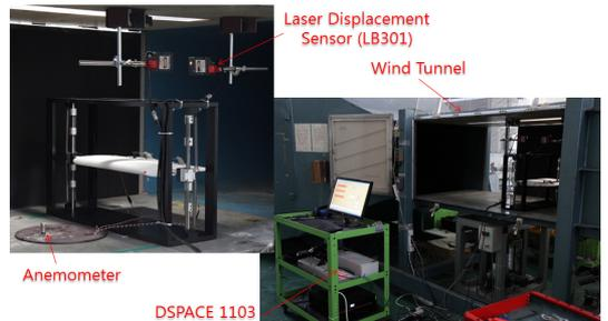
Fig. 9 Wind tunnel test setup
