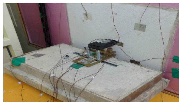
Figure 6. Specimen connecting Panel with Slab by Fastening Unit (Front)
