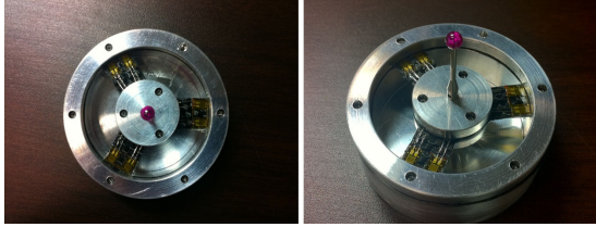
Fig. 5 Prototype of carbon fiber plate force/torque sensor
