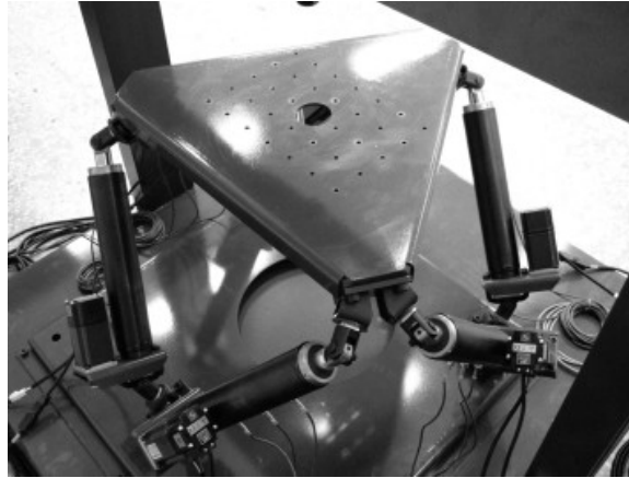
Fig. 1. A 6-SPS pneumatic parallel manipulator.
