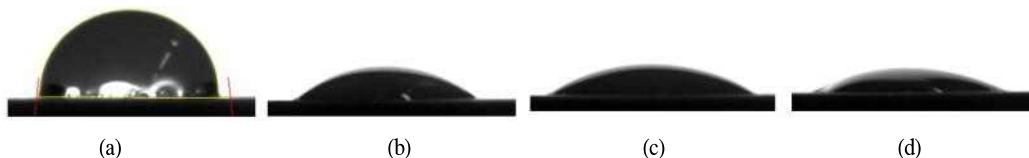
Fig. 3. Distilled water droplet images taken by the video contact angle analyzer (a) disc not immersed, (b-d) discs immersed in NaCl solution for (b)7 days, (c) 14 days and (d) 21 days.
